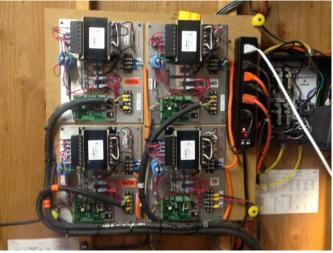
Amplifiers! One for each band! All wall mounted and pre-tuned for each band. Each integrated into the antenna system with Power Output, SWR and status all "touch screen controls"
