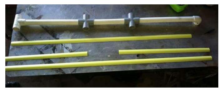
You'll need to cut two pieces of PVC pipe. One piece will be 17 1/2". The other 7". This, along with the PVC connectors, will form the frame of the antenna.
